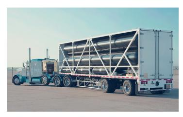
250 bar Hydrogen Mobile Pipeline 350Kg Hydrogen - \$360K
